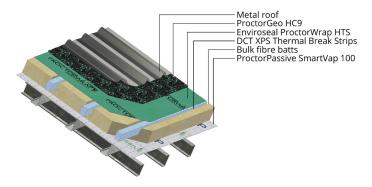
**DCT XPS Thermal Break Strips in Roof**
