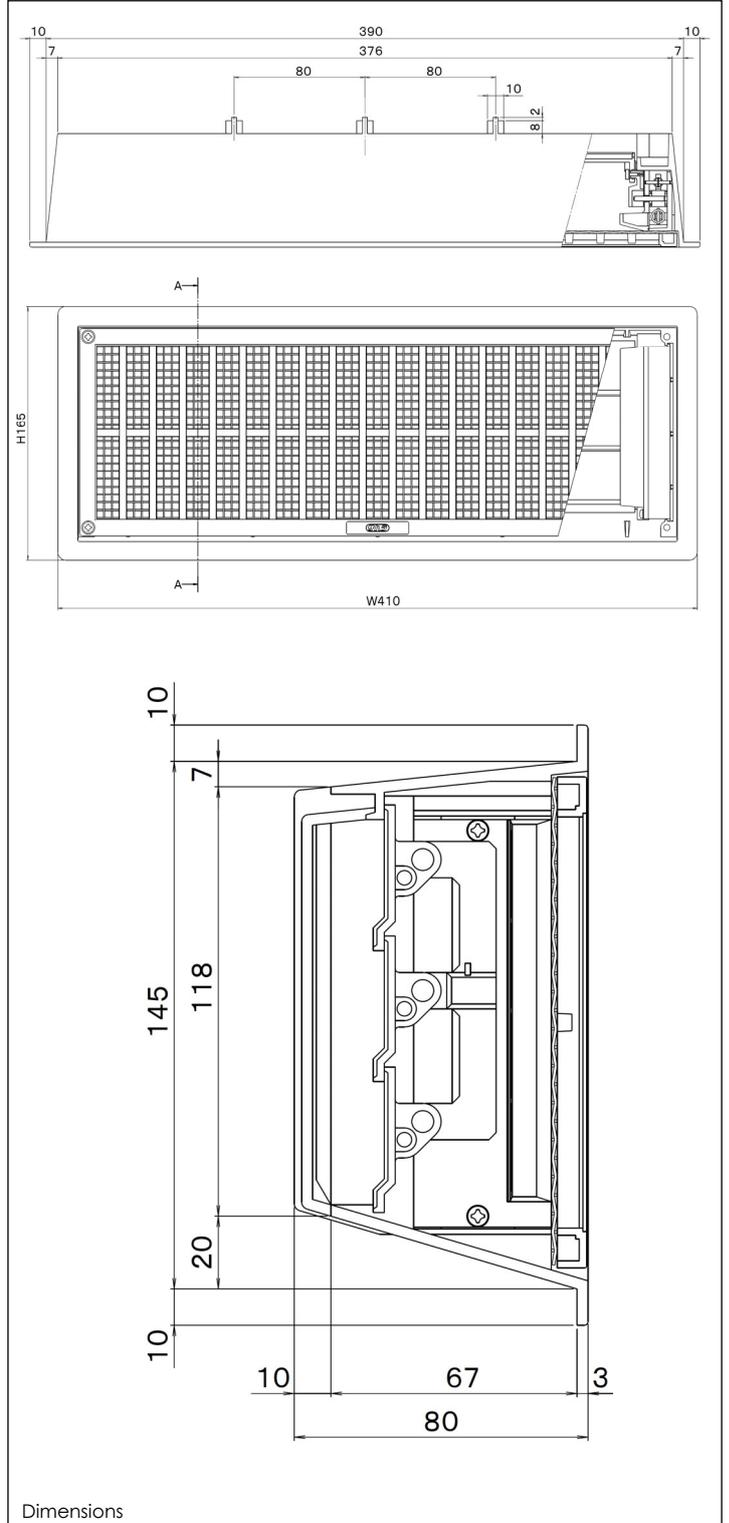
\*Note that the degree of opening may not always reflect the exterior temperature, as this will periodically differ from the ambient temperature where the SMA actuator is located closer to the interior. There is also a lag in adjustment to sharp changes in temperature.
